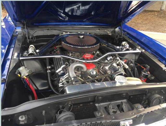
Blocked 302" stroked to 363 cubic inches. The engine is backed up by a built C4 coupled to a 4:11 posi-traction Moser rear end. Frame connectors and traction bars keep it all together with four-wheel disk brakes providing the stopping power. The car is painted Dodge Viper Blue with Viper white racing stripes. At this time I do not have any plans to update the car.
